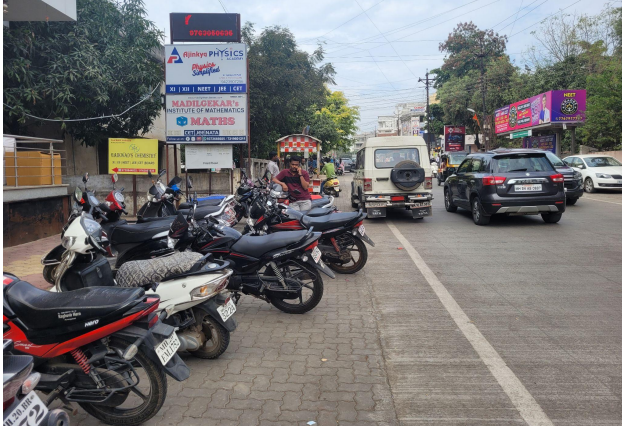
Image 9: Flushed footpath surface being used for Parking
